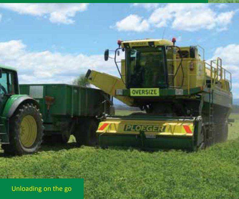
630 mm wide tracks and 5 meter wide new model picking head
