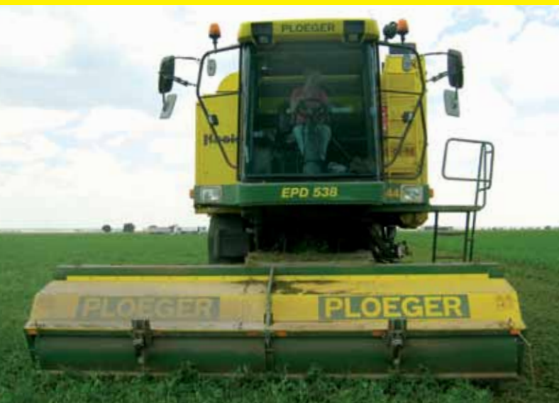
EPD 538 with a 5 meter wide new model picking head w/o ground roller
