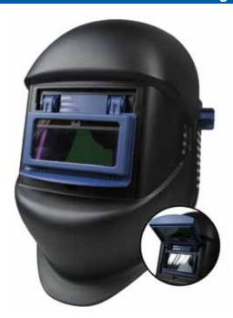
The Multi Vision Xchange is a lightweight Multi Vision welding helmet with unique features. The flip-up holder contains a superior DIN shade-10 automatic cassette with a clear DIN shade-3 neutral position (included). The class 1/1/1/1 cassette in the flip-up holder can at any time be changed for regular welding glass. In other words: this welding helmets offers max. flexibility and a prolonged product lifetime.
