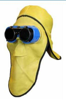
TIG welding mask with flip-up welding goggle and leather face protection of 38 cm. With round welding lenses, diameter of 50 mm shade 10 in flip-up part and, Spectralite anti spatter lenses in flip-up and fixed part.
