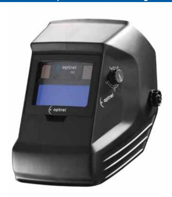
Extra comfortable welding helmet Optrel Solarmatic Comfort (OSC) with automatic colour control from shade 9 till 13. Because of the solar cells there are no on/off switches and battery replacements are not required. a sensorbridge excludes the possible influence of light from other sources. Optrel OSC automatic welding helmets are supplied complete with an unmounted headband. Colour is black.
